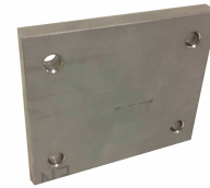
FIGURE 1: Aluminium 6082 T6 plate: 100x90x10 [mm]
