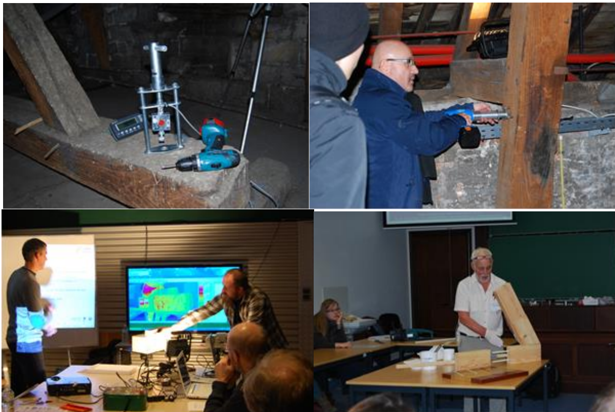
Figure 3: In situ non-destructive testing equipment a) on-site screw withdrawal test, b) on-site core sampling;
