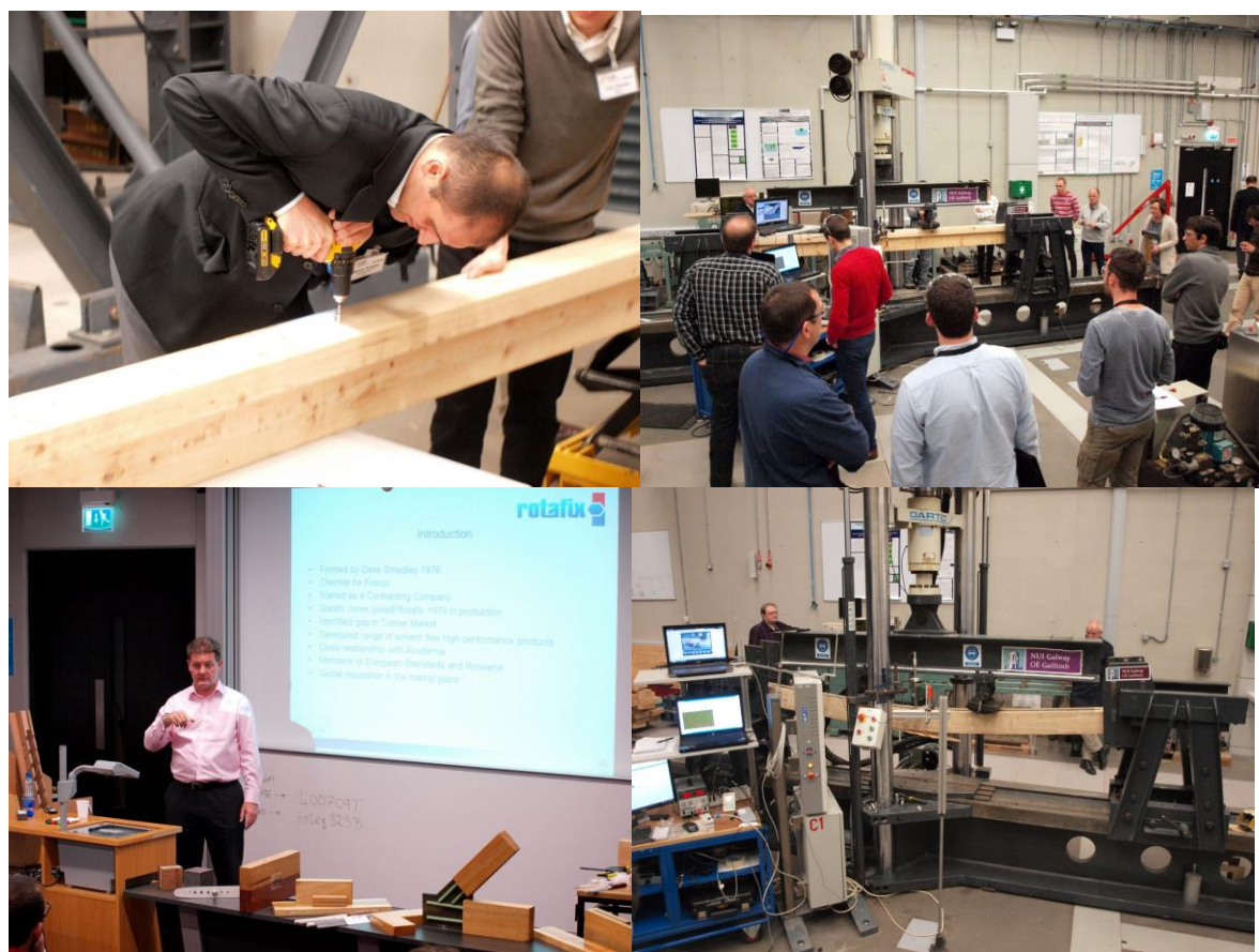
Figure 5 Testing of beams reinforced with self tapping screws and with near surface mounted rods
