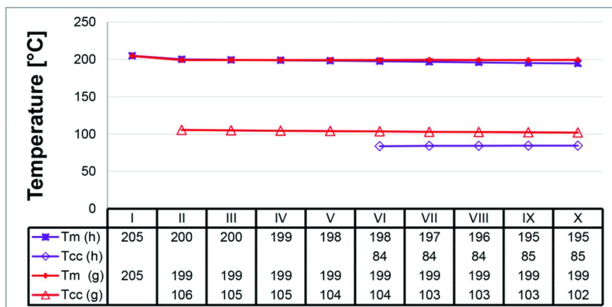
Figure 8. Values of cold crystallization ( T_{cc} ) and melting ( T_m ) temperatures as a function of the heating cycle number (indicated with roman numerals on the top line of the summarizing table under the curve), recorded from the ten cycles DSC thermograms, under nitrogen flow (temperature range: -20 – 230 °C, heating rate 10 °C/min), for the stereocomplex PLA/Cl30B-g-PDLA (5% inorganic, red curves) and Cl30B-g-PLLA/Cl30B-g-PDLA (10%inorganic, violet curves).
