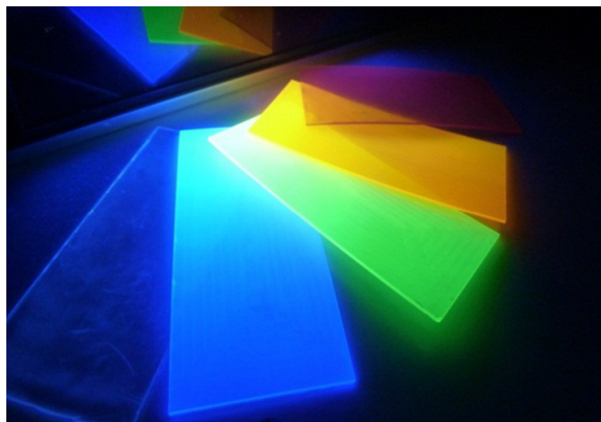
Fig. 6. Plastic scintillators displaying different emission wavelengths (excitation with UV lamp; © CEA) [58].
