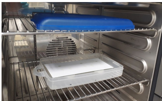
Fig. 2 Incubation system consisted in: a container filled with water, such that the plate did not come into contact with the water, but enough to maintain humidity inside the container when it was covered
