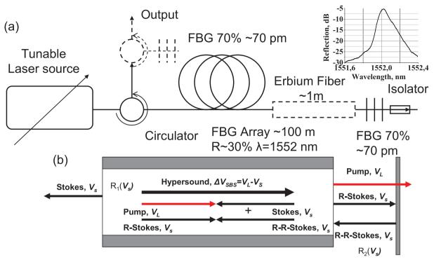
Fig. 1. Experimental setup (a). Interacting waves inside the fiber (b).
