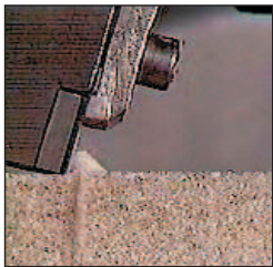
Figure 1 : Picture of the cutter while scratching a sample of Berea sandstone, d = 0.4 mm and drawing of the cutter.
