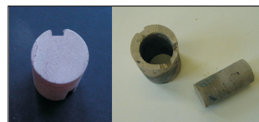
Figure 18 : Test semi-destructive. The sample can undergo other testing after the scratching test.
