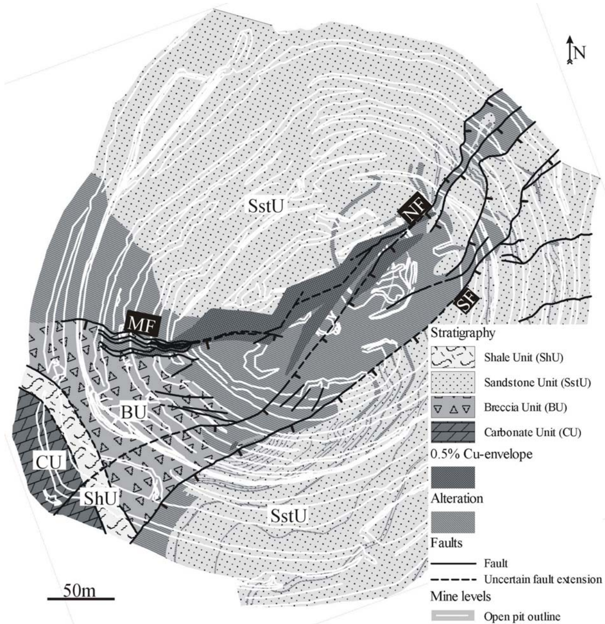
Figure 1. Geological map of the mine showing the stratigraphy, the main fault directions, the 0.5% Cu envelope and the alteration pattern, characterized by a decoloring of the red rocks (SstU=Sandstone Unit, CU=Carbonate Unit, ShU=Shale Unit, BU=Breccia Unit, NF=Northern Fault, SF=Southern Fault, MF=Main Fault Zone).
