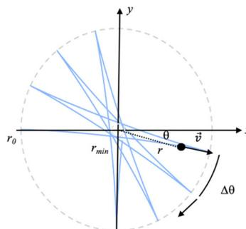
**Figure 3.** Typical trajectory of the FP in the horizontal plane (the pendulum is thus seen from above). The position of the bob is expressed in polar coordinates  $(r, \theta)$  since the bob’s vertical motion is negligible. The shift  $\Delta\theta$  and the instantaneous horizontal velocity  $\vec{v}$  of the bob are displayed. The arrow outside of the circle indicates the direction of the oscillation plane’s rotation viewed from the local frame. Conventions of Figure 2 are kept.
