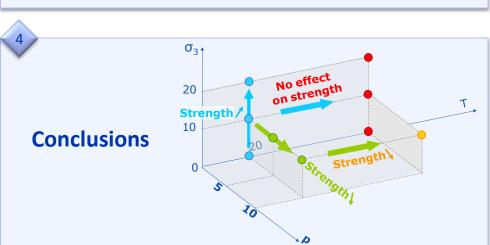
As expected, the strength increases with the confining pressure and decreases with pore pressure. However, whereas no noticeable effect was observed with increasing temperature, a strong coupling is observed by combining both temperature and pore pressure : in fact, for comparable pore pressure, the rock exhibits a strength decrease when the temperature is higher.
