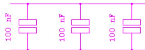
$$C = 100 \text{ nF} + 100 \text{ nF} + 100 \text{ nF} = 300 \text{ nF}$$
