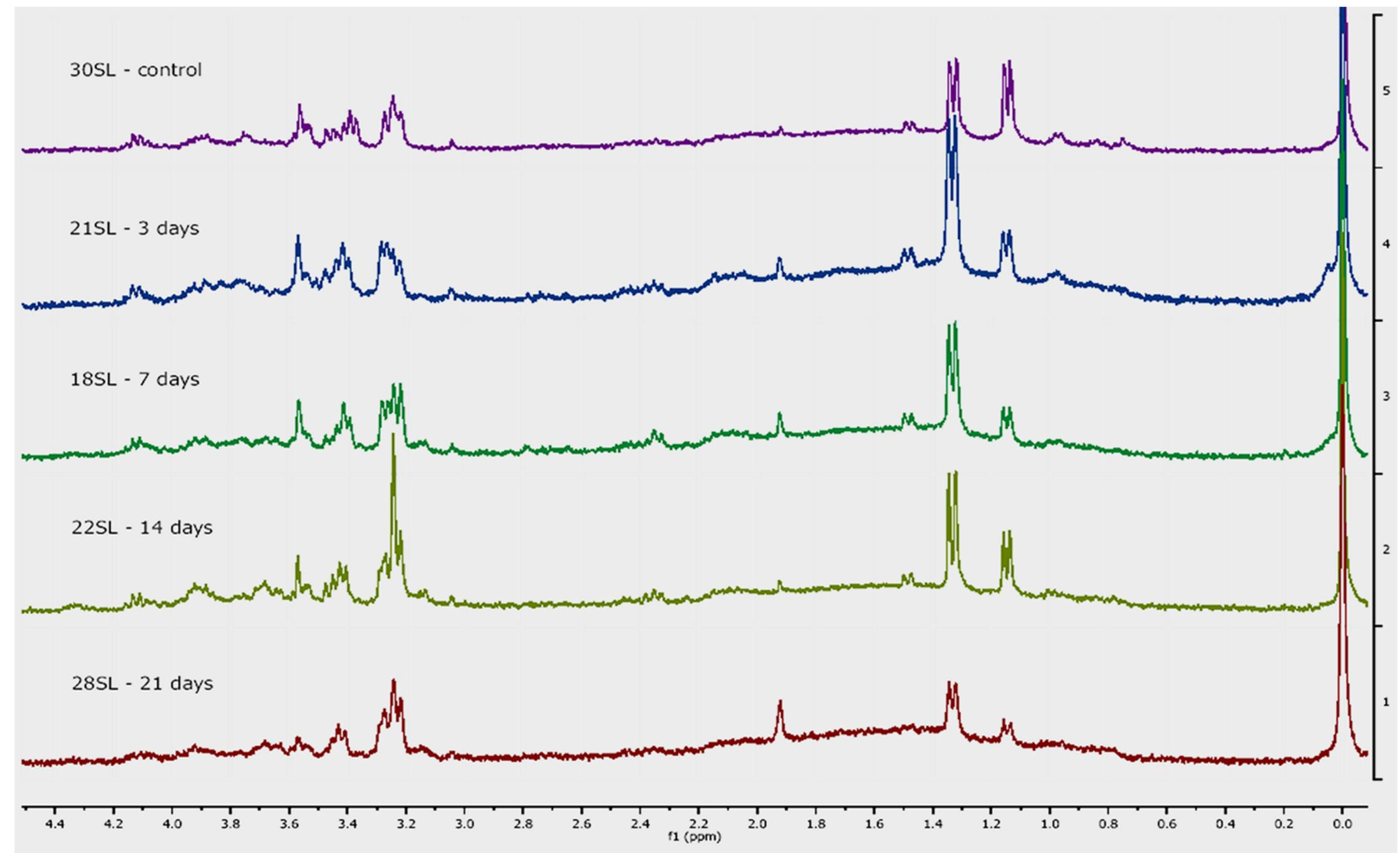
Proton NMR spectra of the aliphatic region of BAL fluid. Time before rat sacrifice is noted close to the spectra.TSP is at 0ppm.
