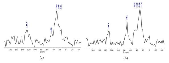
**Figure 5.** <sup>13</sup>C MAS NMR spectra (recovery delay of 0.5 s) of (a) NPFe@FeOx@SiO<sub>2</sub> and (b) NPFe@FeOx@SiO<sub>2</sub>-PEG.
