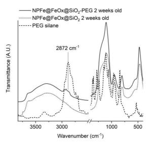
**Figure 4.** DRIFT IR spectra of NPFe@FeOx@SiO<sub>2</sub> (dotted line), NPFe@FeOx@SiO<sub>2</sub>-PEG (solid line), and PEG-silane (dashed line).
