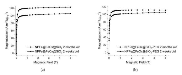
**Figure 6.** Magnetization curves at 37 °C of (a) NPFe@FeOx@SiO<sub>2</sub> and (b) NPFe@FeOx@SiO<sub>2</sub> PEG after 2 weeks and 2 months of retention in water.
