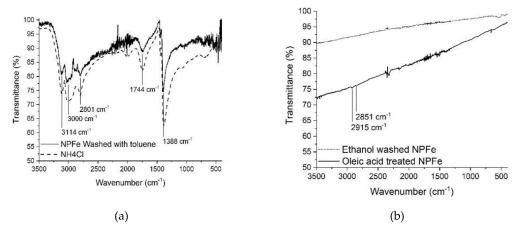
**Figure 2.** FTIR spectra of (a) toluene washed NPFe (solid line) in comparison with  $NH_4Cl$  (dashed line), (b) ethanol washed NPFe (dotted line) and oleic acid treated NPFe (solid line).
