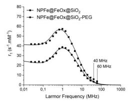
Figure 7. Fitted NMRD profiles of NPFe@FeOx@SiO<sub>2</sub> and NPFe@@FeOx@SiO<sub>2</sub>-PEG.
