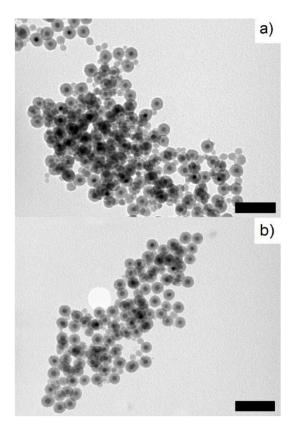
**Figure 3.** TEM micrographs of (a) NPFe@FeOx@SiO<sub>2</sub> and (b) NPFe@FeOx@SiO<sub>2</sub>-PEG. Scale bar: 100 nm.
