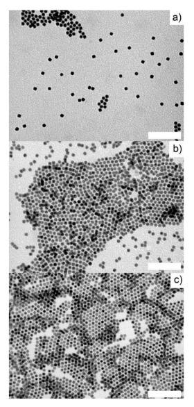
**Figure 1.** TEM images of **(a)** toluene washed zerovalent iron nanoparticle (NPFe), **(b)** ethanol washed NPFe and **(c)** oleic acid treated NPFe. Scale bar: 100 nm.
