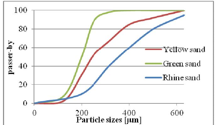
Fig. 6. Graph of passer-by according to particle sizes of sand
