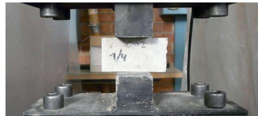
Fig. 3. Compressive test of Rhine sand and white cement
