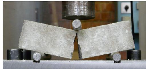
Fig. 2. Bending test of Rhine sand and white cement
