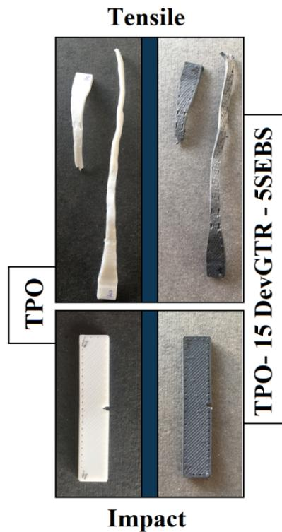
Figure 9. Images of 3D printed specimens after tensile and impact tests.
