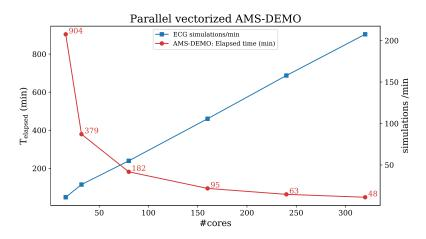
Fig. 2: Strong scaling of vectorized AMS-DEMO on a cluster composed of 108 dual-socket nodes (8-core Xeon E5-2670), using 1, 2, 5, 10, 15 and 20 nodes
