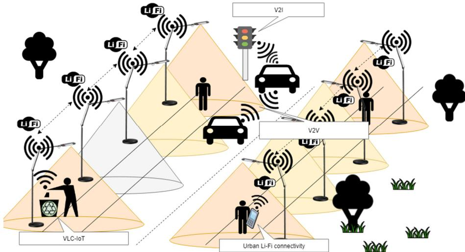
Figure 2. Hypothetic smart city street using VLC technologies.
