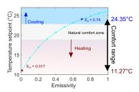
The textile user is comfortable between the lowest setpoint temperature of 11.27 °C and the highest setpoint temperature of 24.35 °C.
