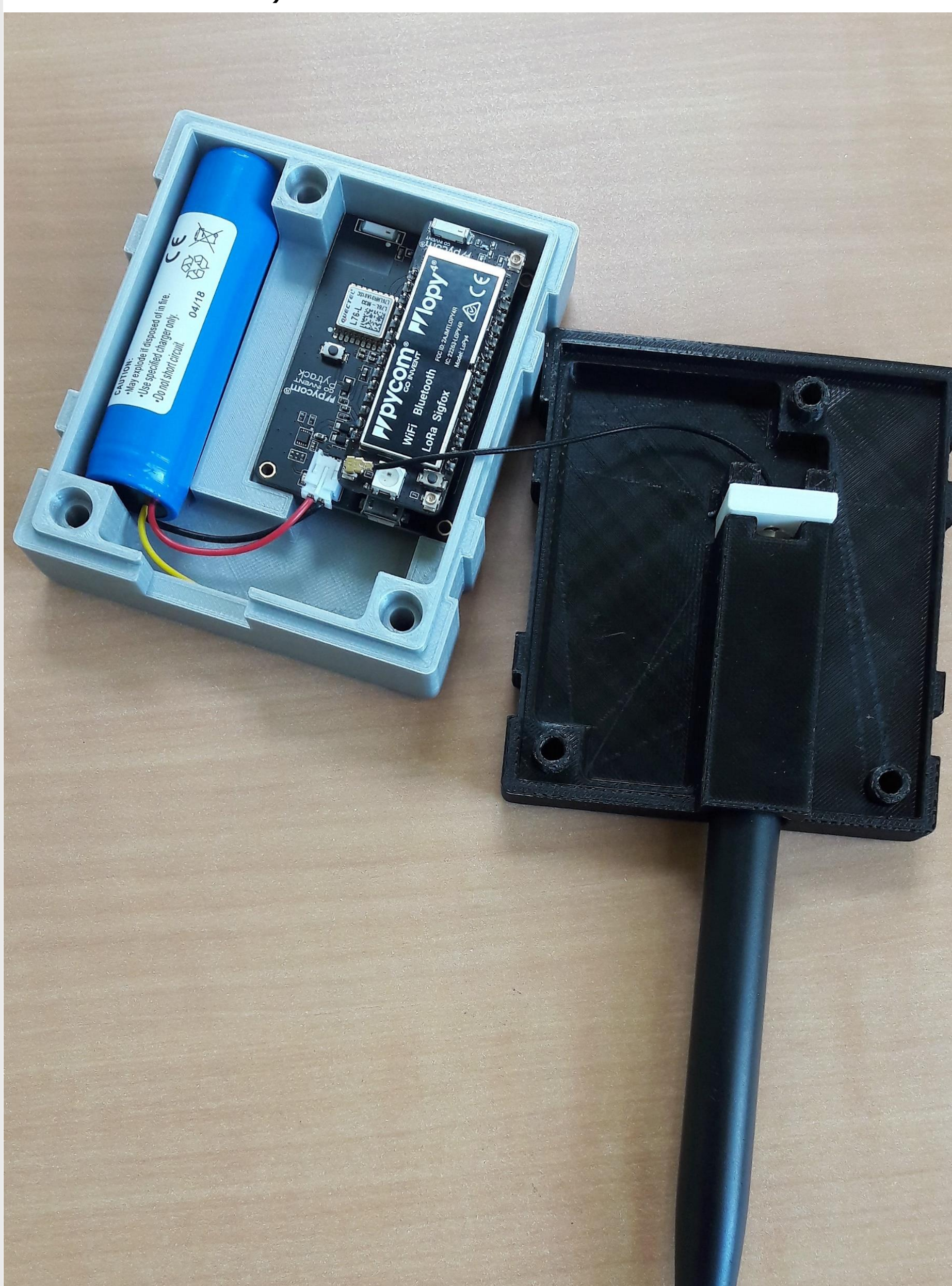
Figure 4: mobile LoRaWAN device with its custom packaging.
