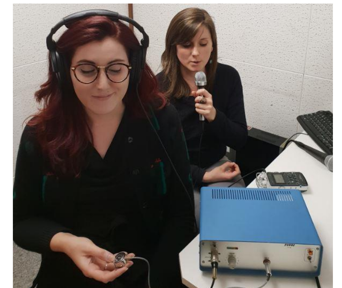
Oral production vibratory amplification and transmission device (Suvag®) Pictures from the UMONS Phonetic Laboratory
