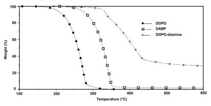
**Figure 1.** Thermogravimetric analyses (TGAs) performed on 9,10-dihydro-oxa-10-phosphaphenanthrene-10-oxide (DOPO), DABP, and DOPO-diamine at 20 °C/min under nitrogen.
