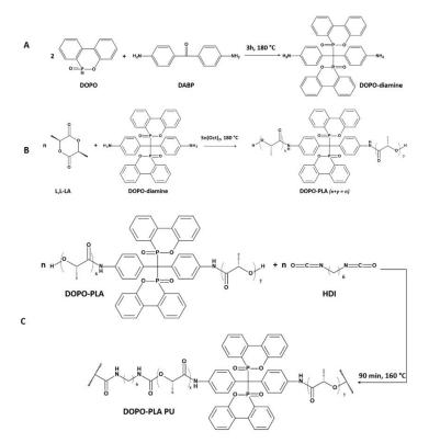
**Scheme 1.** Three-step synthetic pathway to 9,10-dihydro-oxa-10-phosphaphenanthrene-10-oxide (DOPO)-polylactide (PLA) PUs: (**A**) Synthesis of DOPO-diamine; (**B**) DOPO-initiated bulk ring-opening polymerization (ROP) of L,L-lactide (L,L-LA); (**C**) chain coupling reaction.
