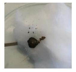
**Figure 9.** Photograph showing the formation of black residue at the surface of cotton after the UL-94 test.
