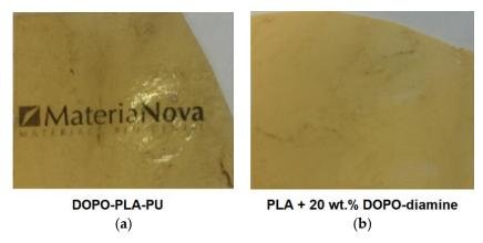
**Figure 6.** Films (thickness of ca. 0.8 mm) of transparent DOPO-PLA-PU (**a**) and the opaque blend of commercial PLA containing 20 wt.% of DOPO-diamine as additive (**b**).
