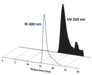
Figure 3. Size exclusion chromatography (SEC) elution curves of DOPO-PLA using both RI and UV detectors.
