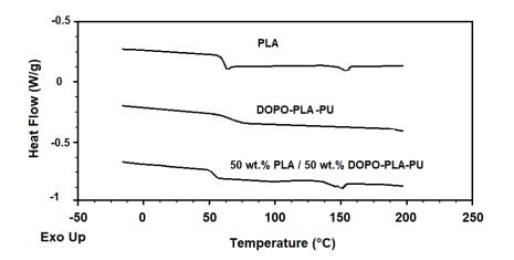
**Figure 7.** Differential scanning calorimetry (DSC) heating curves (second run) of commercially available PLA, DOPO-PLA-PU, and their blend 50/50 (wt/wt.%).
