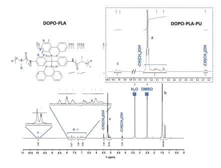
**Figure 5.** <sup>1</sup>H NMR spectrum of DOPO-PLA recorded in DMSO-d6. The figure inset shows the <sup>1</sup>H NMR analysis of DOPO-PLA-PU (only the zoom between  $\delta$  = 4.2 and 10.2 ppm is shown for clarity).
