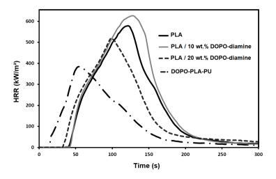
**Figure 8.** Heat release rate (HRR) curves obtained during the mass loss cone calorimeter test at 35 kW/m<sup>2</sup>.
