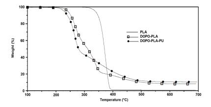
Figure 4. TGA curves of phosphorylated PLA oligomers (DOPO-PLA) and chain extended phosphorylated oligomers (DOPO-PLA-PU) in comparison with commercial PLA, 20 °C/min under nitrogen.
