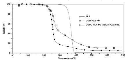
Figure 10. TGA curves under nitrogen (20 °C/min).
