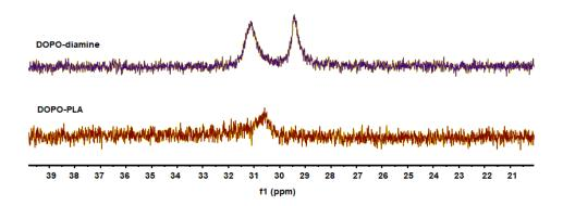
Figure 2. <sup>31</sup>P NMR analyses (zoomed between 40 and 20 ppm) of DOPO-diamine and DOPO-polylactide (PLA)-PU.
