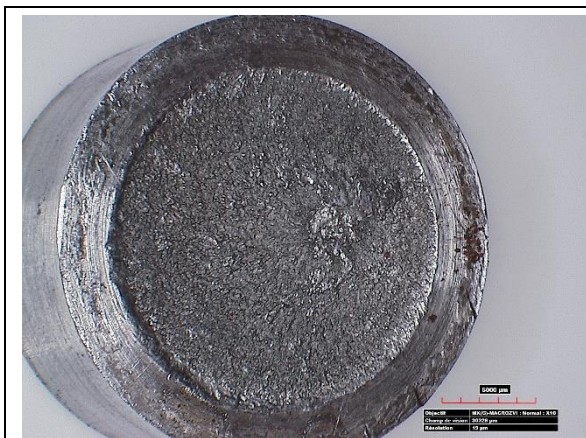
Figure 1. The broken rotating machine shaft
