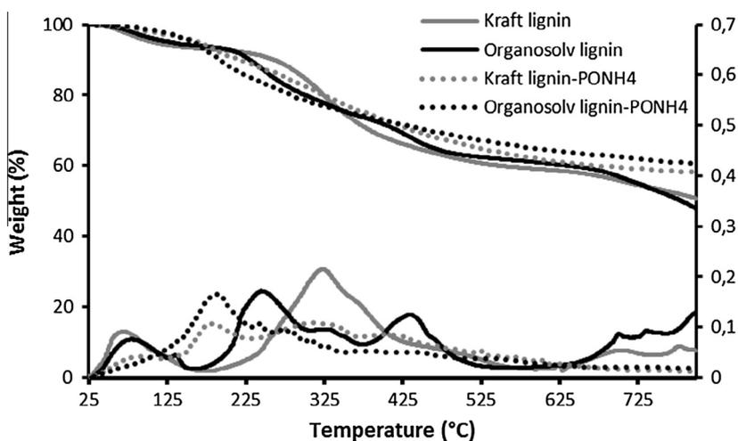
Fig. 3. TG (left axis and upper curves) and DTG (right axis and lower curves) curves of unmodified and modified kraft and organosolv lignins (under N<sub>2</sub>, 20 °C/min).
