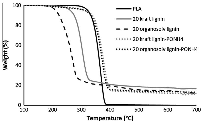
Fig. 9. TG curves of PLA/20 lignin composites compared to the thermal behavior of neat PLA (under  $N_2$ , 20 °C/min after 10 min of isothermal at 100 °C).
