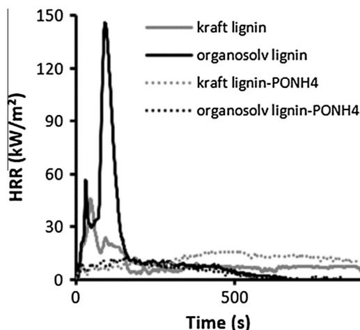
Fig. 5. HRR curves of untreated and treated kraft and organosolv lignins.
