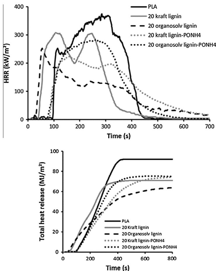
Fig. 10. HRR and THR curves of neat PLA and PLA/20 lignin composites.
