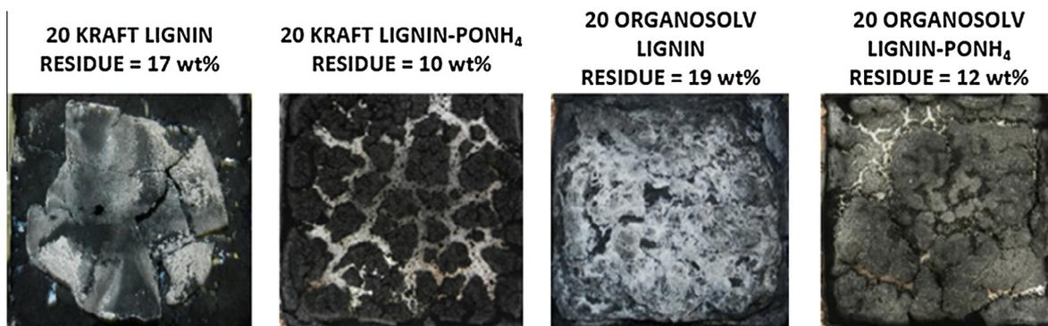
Fig. 11. Pictures of the residues of combustion of PLA/20 lignin composites.
