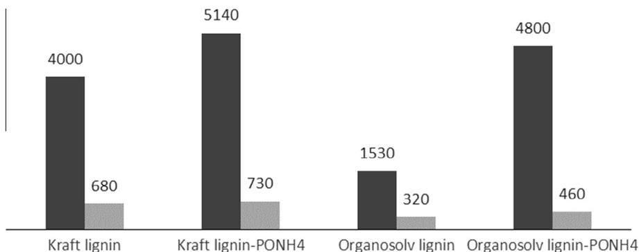
Fig. 2. Average molecular weight (in Da) of unmodified and modified Kraft and Organosolv lignins.
