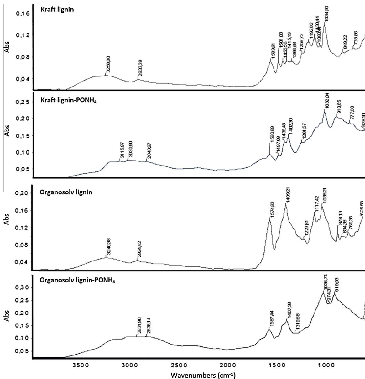
Fig. 1. Infrared spectra of unmodified and modified kraft and organosolv lignins.
