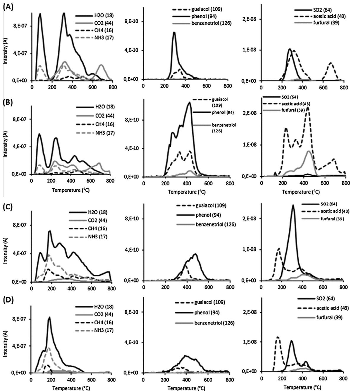
Fig. 4. Gases released during thermal degradation of kraft lignin (A), organosolv lignin (B), kraft lignin-PONH4 (C) and organosolv lignin-PONH4 (D) under N<sub>2</sub>.
