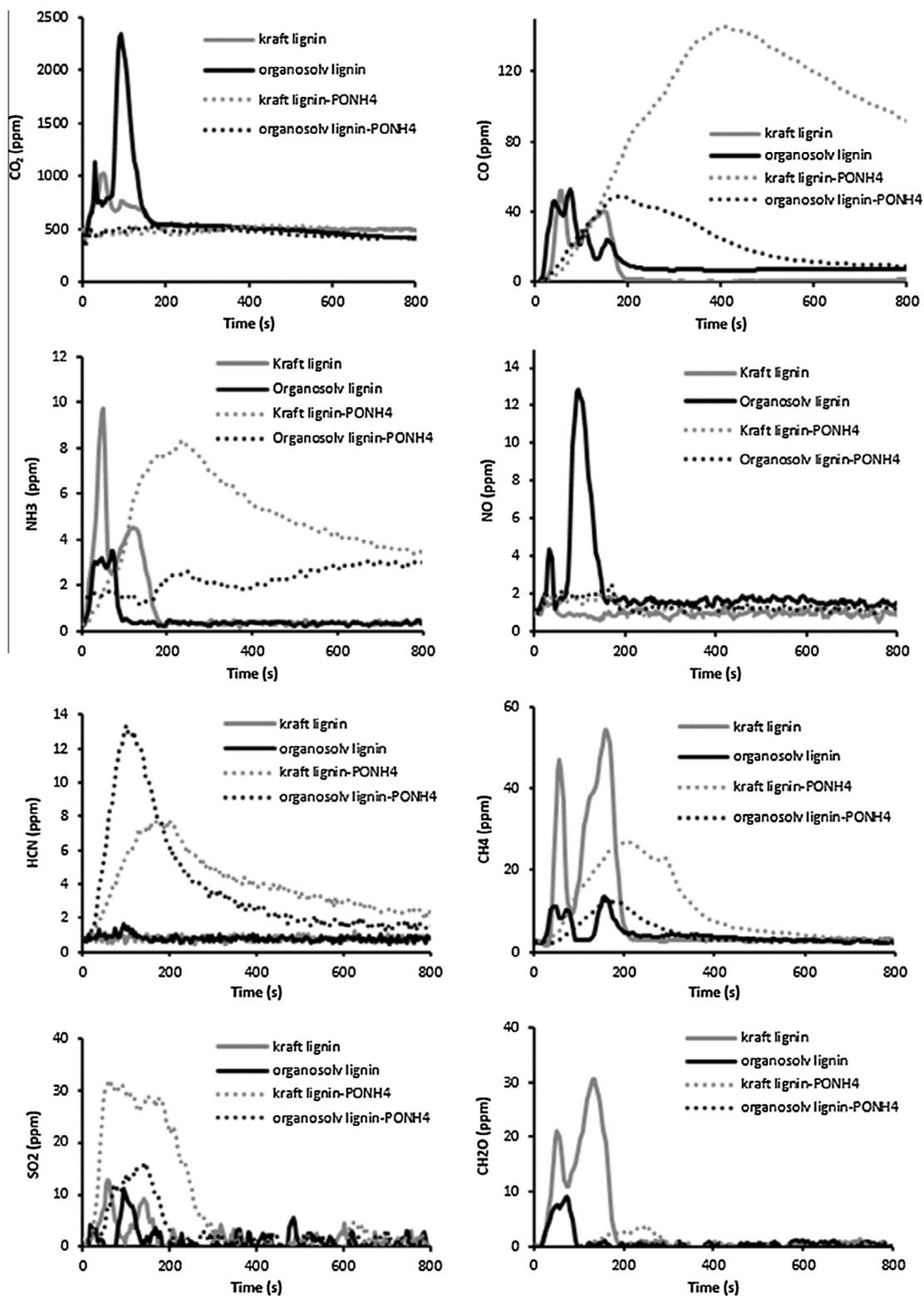
Fig. 7. Composition of the smokes in CO<sub>2</sub>, CO, NH<sub>3</sub>, NO, HCN, CH<sub>4</sub>, CH<sub>2</sub>O and SO<sub>2</sub> of kraft and organosolv lignins (untreated and treated).
