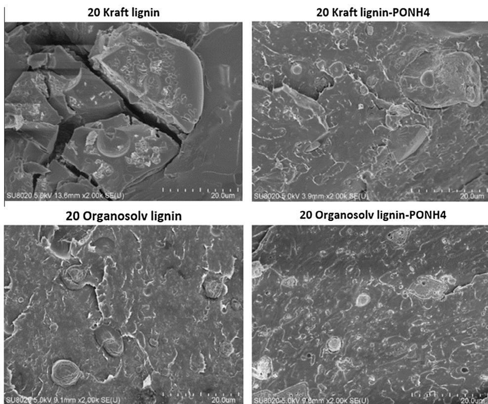
**Fig. 8.** SEM pictures of PLA/20 lignin composites. Effect of the lignin type (kraft or organosolv) and chemical functionalization via ammonium phosphate grafting reaction.
