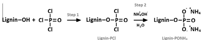
Scheme 1. Two-step chemical modification of lignin.
