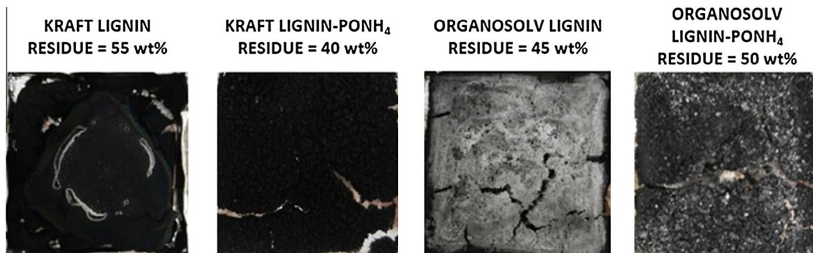
Fig. 6. Pictures of the residues obtained after cone calorimeter test.
