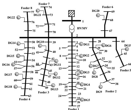
Fig. 2. 77-bus radial distribution system
