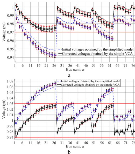
**Fig. 9.** The voltages obtained using simplified network component models as well as boxplots of initial and corrected voltages considering the uncertainties associated with the load, line, and transformer models (a) in the voltage drop case, (b) in the voltage rise case
