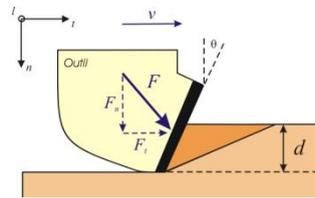
Figure 2: scratching test setup
