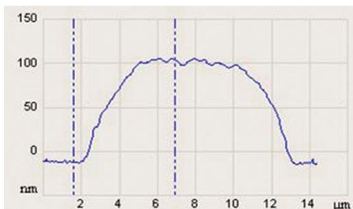
Fig. 2 TM-AFM height profile over one dot PDMAEMA.
