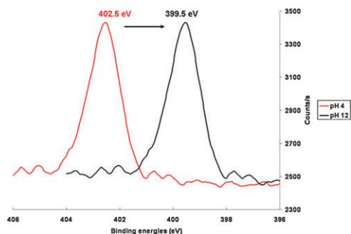
Fig. 3  $N_{1s}$  XPS spectrum of PDMAEMA brushes under acidic and alkaline conditions.
