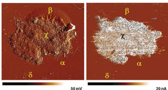
**Fig. 5**  $20 \times 20 \mu\text{m}$  AFM images in deflection mode (left) and current (right). ( $\alpha$ ) Self-assembled thiol- $\text{CH}_3$  layer on gold surface; ( $\beta$ ) partially uncovered PDMAEMA brushes; ( $\delta$ ) isolated CNTs on the thiol- $\text{CH}_3$  layer; ( $\gamma$ ) CNTs on PDMAEMA brushes.
