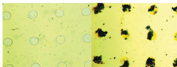
Fig. 4 Microscopic view (magnification 50 $\times$ ) of the naked PDMAEMA pattern (left) and after selective anchoring of CNTs on polymeric brushes (right). (Circular pattern diameter: 10  $\mu$ m.)
