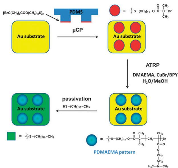
**Fig. 1** Schematic representation of thiol derivative deposition by  $\mu$ CP on a gold surface, synthesis of PDMAEMA brushes by ATRP and passivation of the gold substrate.
