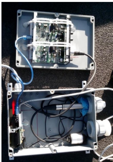
Figure 5: The Electronics Box, with Sound Card Fixed to the Top and no SIM Dongle yet.
