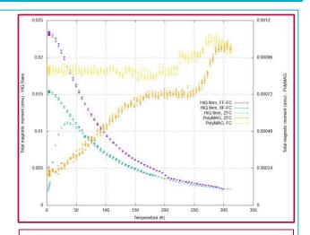
Magnetic measurements at 5mT from a two samples, obtained following various experimental protocols: ZFC, classic FC (FF-FC), and FC after freezing the sample under zero field and then switching on the field (OF-FC).
