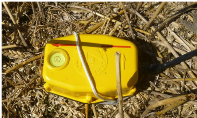
Fig. 4. In-field deployment of a three component geophone.
