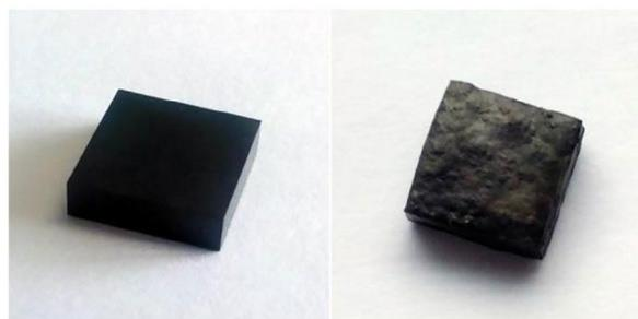
**Figure 3** Illustration of the sample shape preservation on a sample of  $1 \text{ cm}^2$ . Left: before pyrolysis, right after a pyrolysis at  $1000 \text{ °C}$  under  $\text{N}_2$
