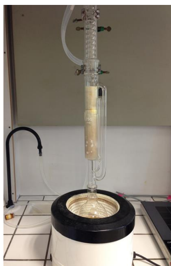
Figure 3.3: The Soxhlet extraction applied to a poultry sample in our lab.
