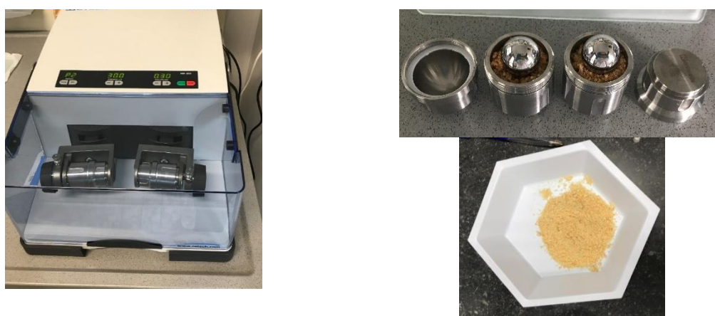
Figure 4.2: Mixer mill MM400 by Retsch that offers efficient grinding for small samples by impact and friction. 10 g of sample were put in each grinding jar with metallic balls. Rapid radial oscillations in a horizontal position of the grinding jars, combined with the movement of the balls, resulted in a thorough milling of samples.
