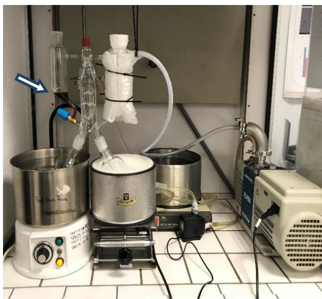
Figure 3.4: View of the assembled equipment for SAFE, the temperature of the water in the left leg and the head is 30°C, ensured by water inlet. The left vessel is incubated in a water bath at 40°C; on the other side, the trap and right vessel are cooled by liquid nitrogen at -196°C. The arrow indicates the vessel in which the sample is introduced (original image).
