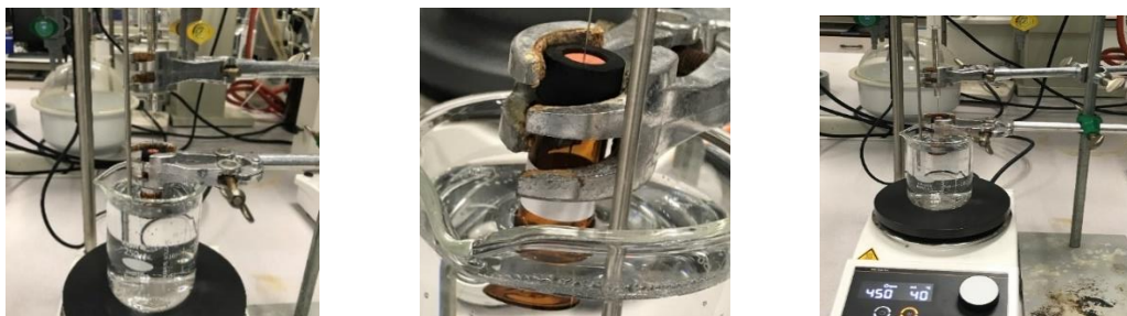
Figure 3.7: HS-SDME application, the vial containing the sample and magnetic rod is placed in a water bath at 40°C; stirring speed, 450 rpm; volume of suspended PFBHA in heptane from the micro syringe, 3 \mu L (original images).
