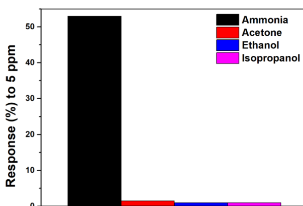
Figure 12. Selectivity test: Response of PPy sensors after reduction treatments in \text{Na}_2\text{SO}_3 10 wt% solution in demineralized water to 5 ppm ammonia, acetone, ethanol, and isopropanol.
