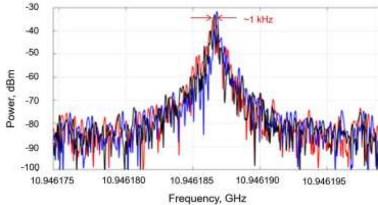
Fig. 4. RF frequency drift for 10 minutes.
