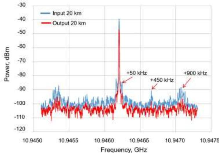
Fig. 5. Spectrum of the carrier signal and its harmonic components at the 20 km optical fiber input and output.
