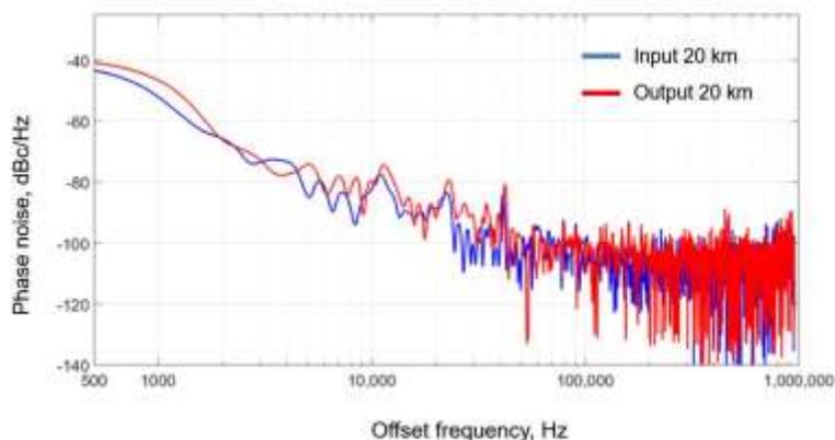
Fig. 6. Phase noise at the input and output of the 20 km optical fiber.
