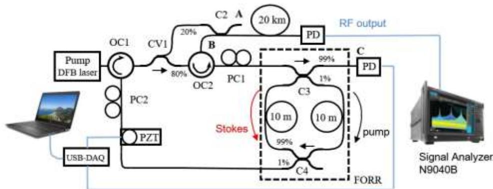
Fig.1. Experimental setup: USB-DAQ – microcontroller, PD – photodetector, OC- optical circulator, PC – polarization controller, CV1 – variable coupler, C – coupler, PZT-fiber piezo stretcher, FORR – fiber optic ring resonator.
