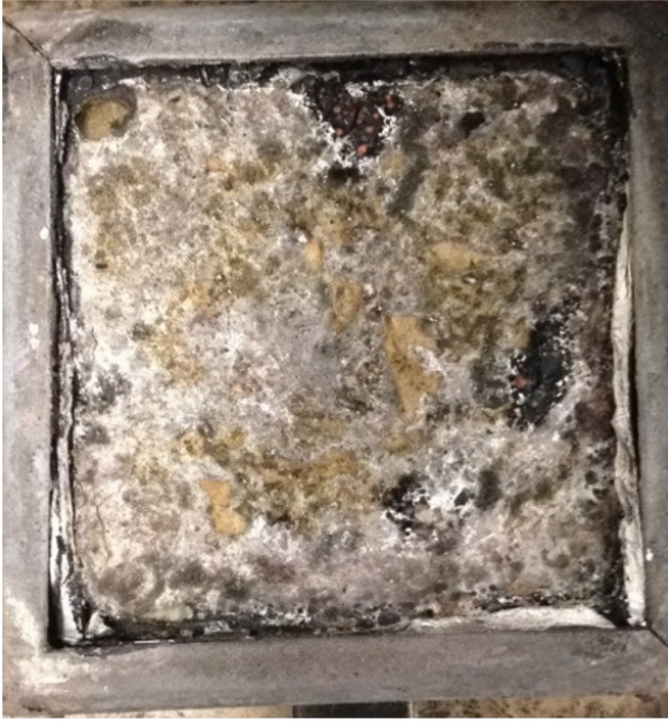
Figure 4: Picture of the final residue after cone calorimeter test of EVA containing 60 wt% unmodified lignin
