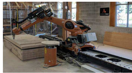
Figure 2.22: Additional linear axis [38]
