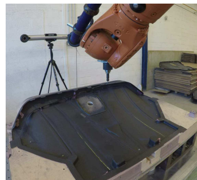
Figure 2.16: Carbon fiber trimming [32]
