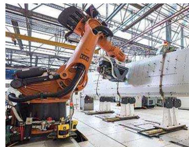
Figure 2.14: Drilling of aerospace parts [30]
