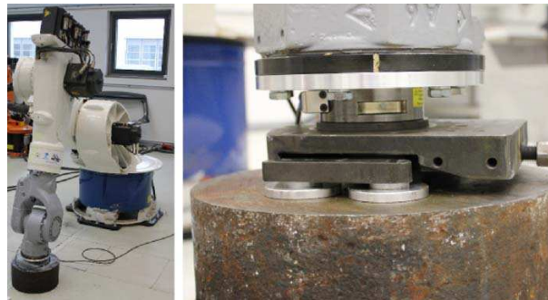
Figure 2.30: Clamping of the end-effector for stiffness identification [61]
