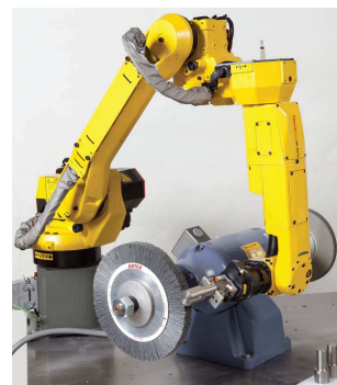
Figure 2.20: Polishing of a carried part [36]
