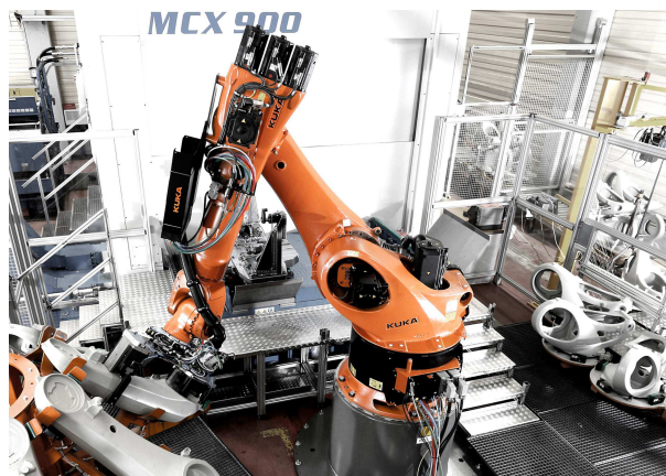
Figure 2.10: Kuka robot KR Quantec milling parts in its own production [13]
