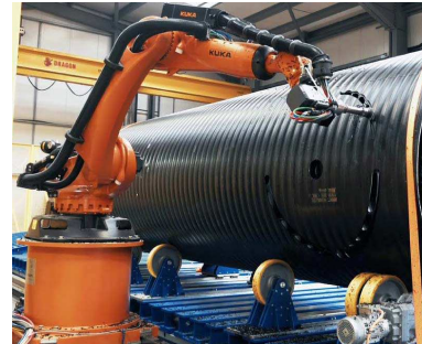
Figure 2.15: Milling of gigantic pipe [31]
