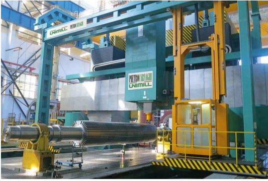
(a) Milling of rotor for power plant generator [11]
