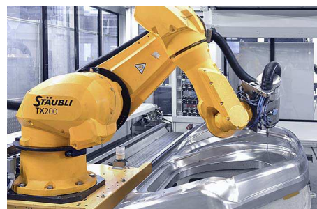
Figure 2.17: Mould drilling for Audi [33]
