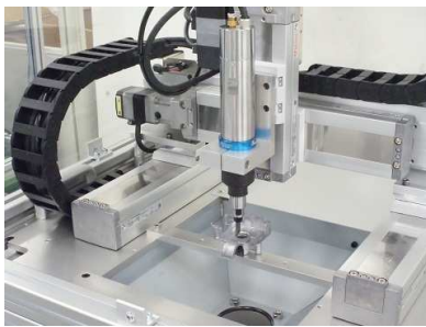
(a) Deburring of metal parts with a Cartesian robot [8]
