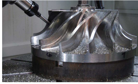
Figure 2.1: Milling of a centrifugal impeller [2]
