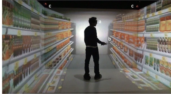
Figure 2.4: A CAVE-like setup used to create a virtual grocery store. Reproduced from (Borrego et al., 2016).
