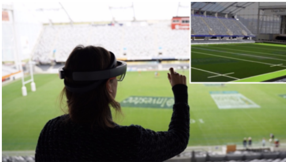
Figure 2.10: An AR feature to superimpose virtual line marks on a rugby field, through a HoloLens headset. Reproduced from (Zollmann et al., 2019).
