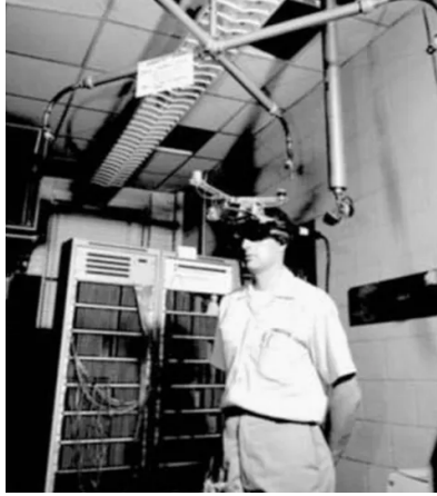
Figure 2.7: The sword of Damocles. A mechanical tracking system designed for an early HMD. Reproduced from (Sutherland, 1968).
