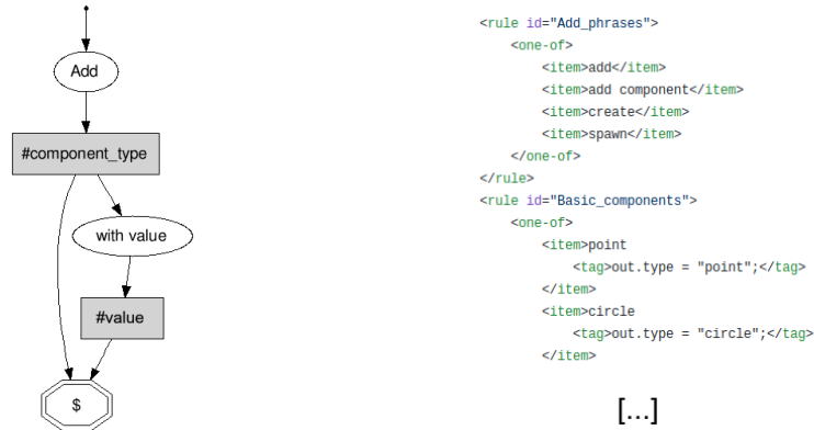
(a) A visual representation subsuming the grammar rules used to add components. (b) Part of the corresponding definition in the XML-based SRGS format.
