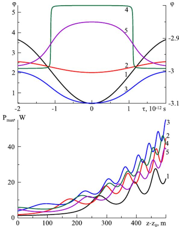
**Fig. 6.** (a) Time dependence of the pulse phase at the input of the inhomogeneous fiber section and (b) the distribution of the maximum pulse power over the inhomogeneous fiber length (b) calculated for different lengths of the homogeneous fiber section:  $z_0 = (3; 4; 5; 5.65; 6) \cdot 10^2$  m — curves (1; 2; 3; 4; 5).
