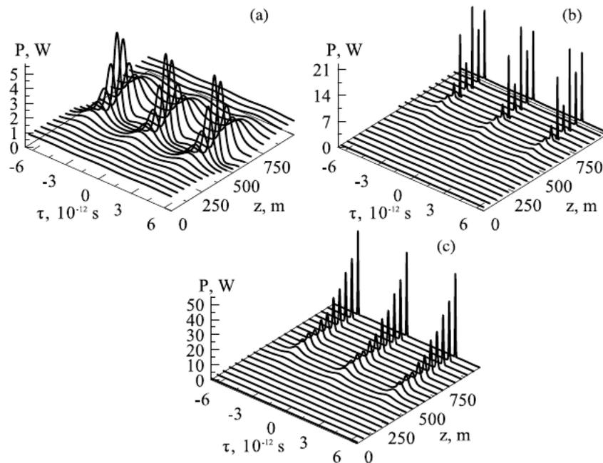
Fig. 5. Evolution of a weakly modulated ( $m = 0.01$ ) continuous wave calculated in the homogeneous (a) and inhomogeneous (b) passive optical fibers and in a passive two-cascade fiber configuration (c) calculated for the input power of  $P_0 = 1 \text{ W}$ , modulation frequency  $\Omega_{\text{mod}} = \sqrt{2RP_0/|D_0|}$ ,  $z_0 = 500 \text{ m}$  and  $b = 5 \cdot 10^{-3} \text{ m}^{-1}$ .
