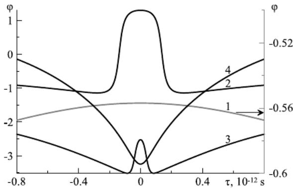
Fig. 4. Temporal phase profiles of the modulated continuous wave calculated for different  $b$  values:  $b = (0, 3, 5, 7) \cdot 10^{-3} \text{ m}^{-1}$  (curves 1–4),  $P_0 = 1 \text{ W}$ ,  $L = 1000 \text{ m}$ .
