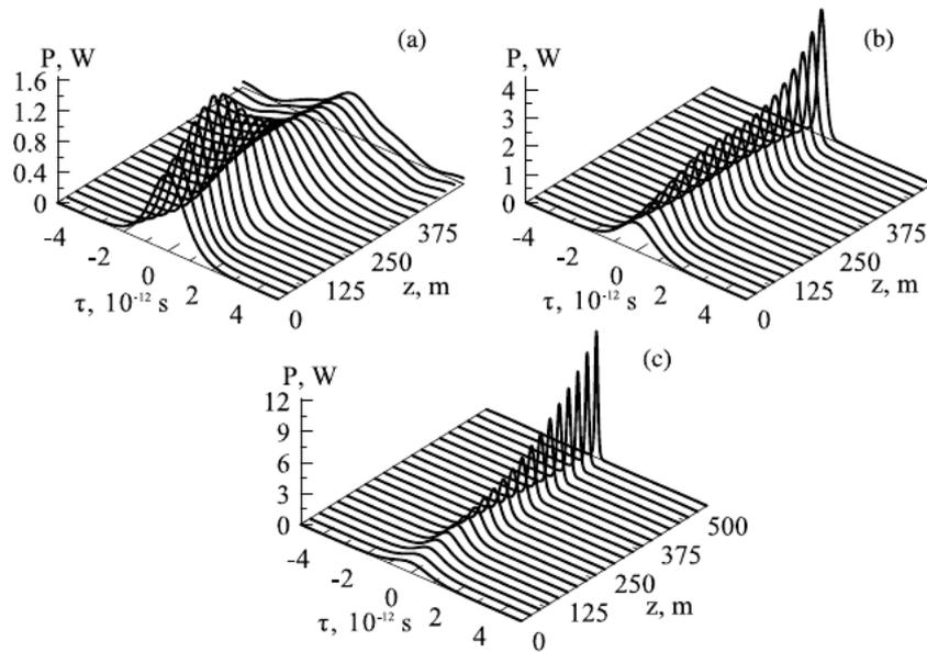
Fig. 1. Pulse evolution in the inhomogeneous fiber calculated for  $R_0 = 10^{-2} \text{ W}^{-1} \text{ m}^{-1}$ ,  $D_0 = -10^{-26} \text{ s}^2 \text{ m}^{-1}$ ,  $b = (0, 3, 5) \cdot 10^{-3} \text{ m}^{-1}$  (a, b, c),  $\alpha_0 = 2.5 \cdot 10^{23} \text{ s}^{-2}$ ,  $\tau_0 = 10^{-12} \text{ s}$ ,  $P_0 = 1 \text{ W}$ .
