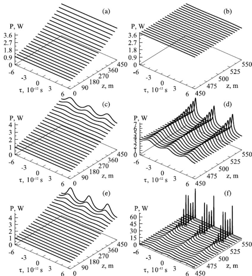
**Fig. 8.** Evolution of a weakly modulated ( $m = 10^{-4}$ ) WP in a two-cascades fiber configuration comprising homogeneous active (a, c, e) and in homogeneous passive (b, d, f) optical fibers simulated for  $b = 2.5 \cdot 10^{-2} \text{ m}^{-1}$  (b; c; d) and  $\Delta\omega_L = (0.1; 1; 10) \cdot 10^{12}$  (a; b; c; d; e, f). Other parameters are the same as in Fig. 7.
