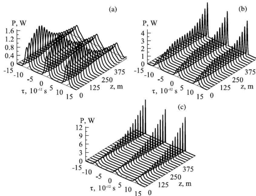
Fig. 2. Pulse train evolution in the inhomogeneous passive fiber. The pulse period is  $T = 5\tau_0$ . Other calculation parameters are the same as in Fig. 1.
