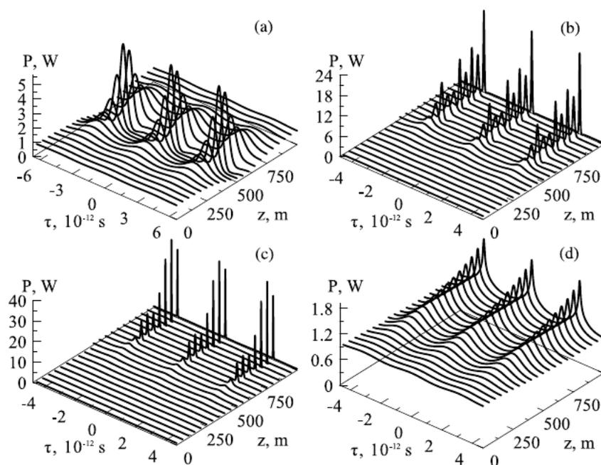
Fig. 3. Evolution of weakly modulated ( $m = 0.01$ ) continuous wave calculated for different  $b$  values:  $b = (0, 3, 5, 7) \cdot 10^{-3} \text{ m}^{-1}$  (a, b, c, d),  $P_0 = 1 \text{ W}$ .
