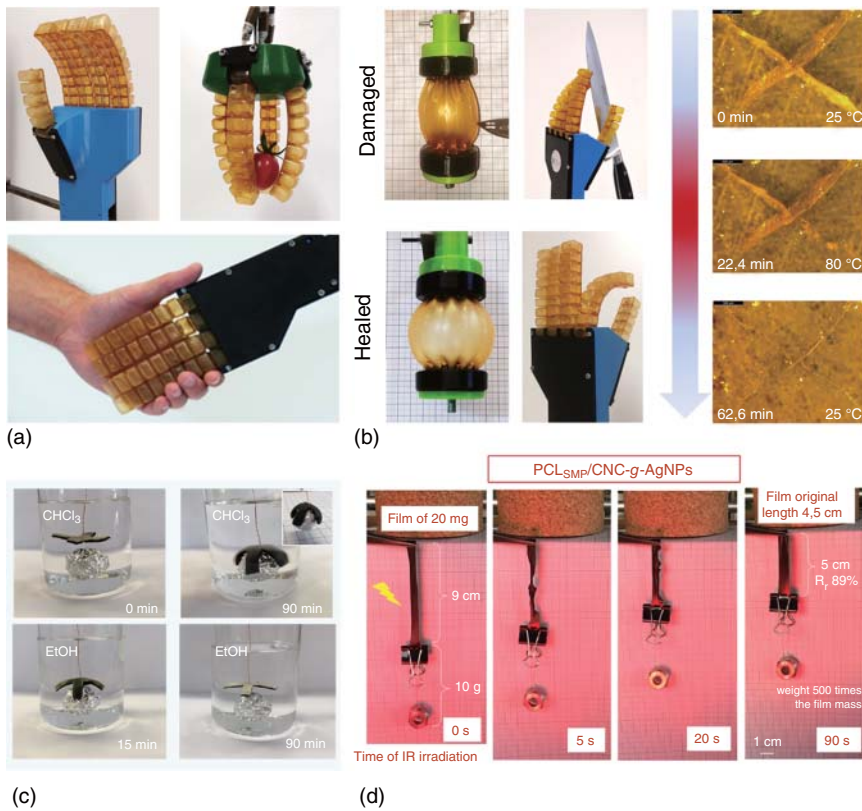
Figure 11.10 Soft robotic DA-based thermo-reversible networks with self-healing properties (a and b) and for object catching and transportation upon solvent (c) or remote IR light (d) actuation. Source: (a and b) Terryn et al. 2017 [107]. Adapted with permission of Science Robotics. (c) Toncheva et al. 2017 [109]. Adapted with permission of RSC. (d) Toncheva et al. 2018 [110]. Adapted with permission of ACS.
