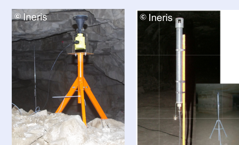
Radar and microphone as permanent monitoring devices in the Hellemmes quarry (FR)
