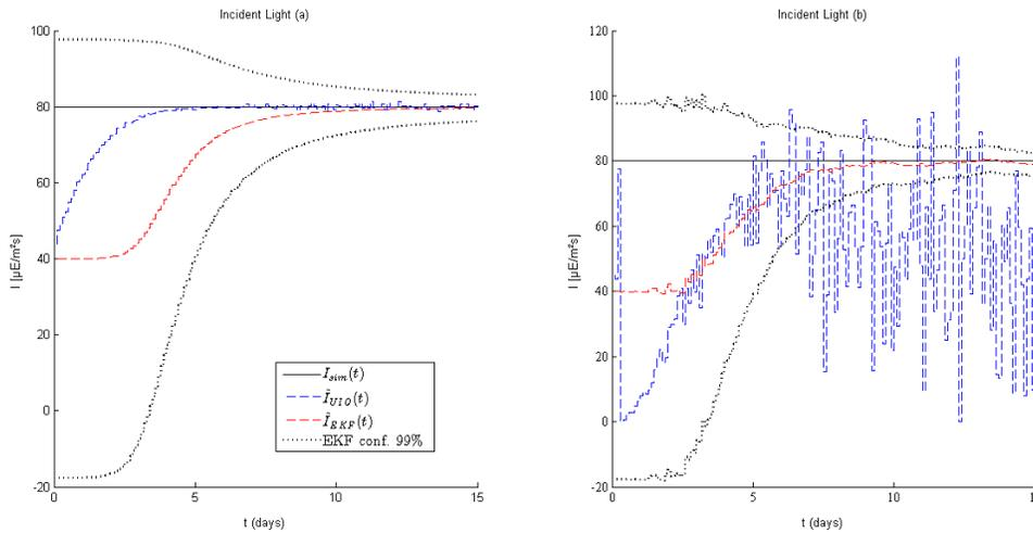
**Figure 3.** Incident light estimation with EKF and UIO (a) low noise level (b) higher noise level on measurements
