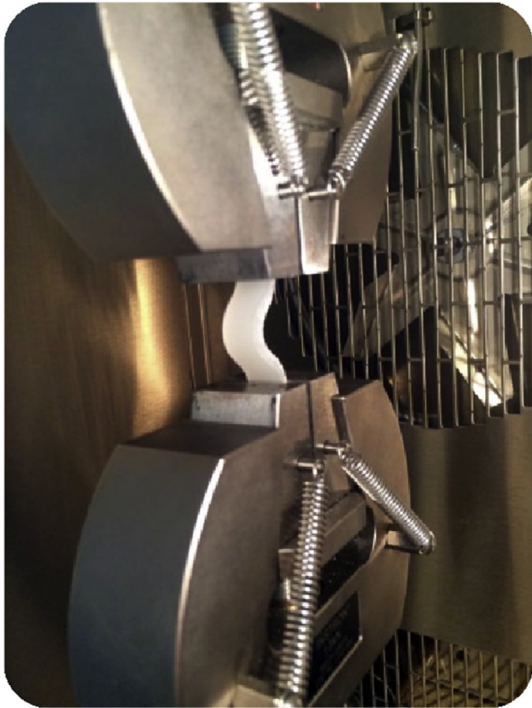
Fig. 8. Buckling of PLA-BS specimen during cyclic loading at 20 Hz and 60 °C.
