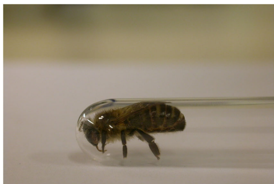
Fig. 1 Lyophilized honey bee in a quartz tube for EPR imaging analysis
