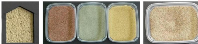
Figure 5: target mortar (left), available sands (centre), obtained mix (left)
