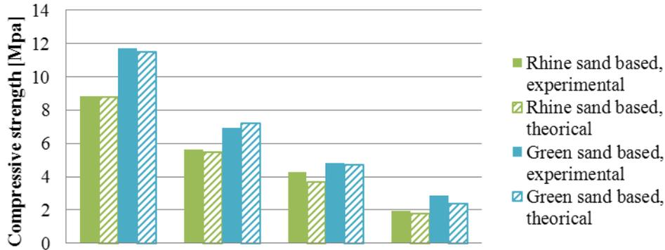
Figure 4: compressive strength (prediction | measure) for various mortars
