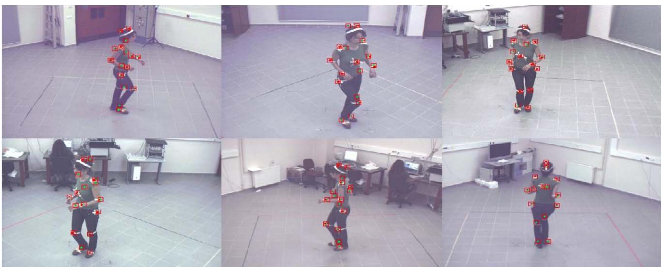
Fig. 4 An example scene from the 3D joint positions tracking process. Red pixel regions in the red search windows represent the marker candidate pixels for the current frame. Green dots are the 2D projections of the 3D marker positions for the previous frame
