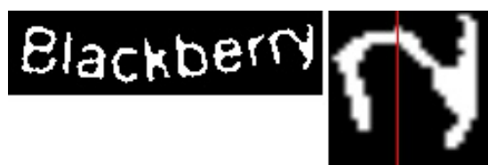
Figure 9: Left: A word with touching characters. Right: Caliper algorithm: the chosen cut (in red) between “r” and “y” of the “Blackberry” word.
