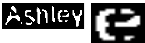
Figure 8: Left: broken characters in a street name. Right: overlap of four parts of the character “e”.
