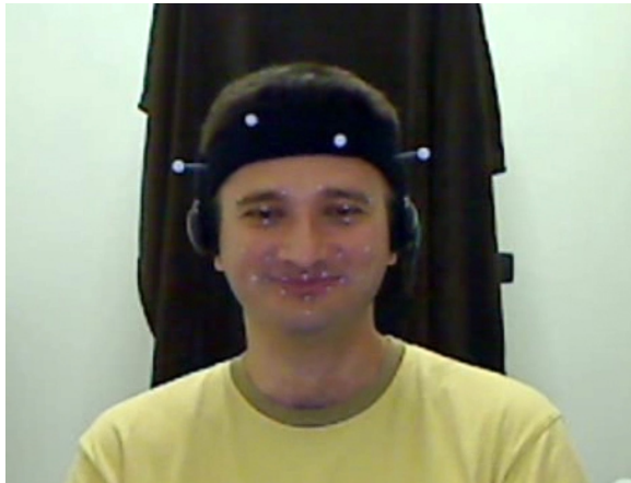
Figure 2.2: Infrared markers placed for facial motion tracking using OptiTrack.
