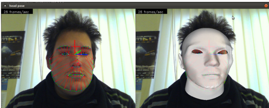
Fig. 3. On the left we have the face tracking and on the right the projection of the 3D model is correctly superposed on the points from the face tracking. The whole system works in real-time.
