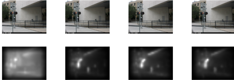
Figure 1.2. Illustration of the GBVS method: on the first row: 4 frames of a video sequence, on the second row: the corresponding saliency maps. Inspired by [3].
