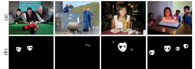
Fig. 4. Applying face detection method from [15]. (a) Input images, (b) Result of face detection. The results contain either big faces (brighter), either small faces, and either both big and small faces.
