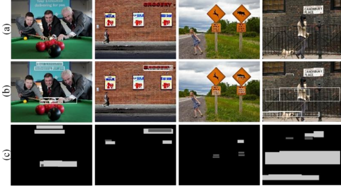
Fig. 5. Applying text detection method from [14]. (a) Input images, (b) Result of text detection inside white bounding boxes, and (c) Converting text detection areas into white to indicate text features. The results contain both big (brighter) and small texts.
