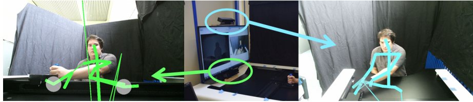
Fig. 11. Comparison of the view from the kinect below (green) and above the screen (light blue).
